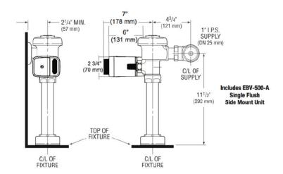
**NOTE:** All vitreous china dimensions shown in these drawings are nominal. Dimensions can vary within the tolerances established in the governing ASME A112.19.2/CSA B45.1 standard. Please take this into consideration when planning rough-in and plumbing layouts.
