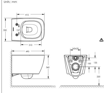
**Note:**-All vitreous china dimensions shown in these drawings are nominal. Dimensions can vary within the tolerances established in the governing BIS standard. Please take this into consideration when planning rough-in and plumbing layouts.
