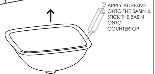
APPLY ADHESIVE ONTO THE BASIN & STICK THE BASIN ONTO COUNTERTOP
