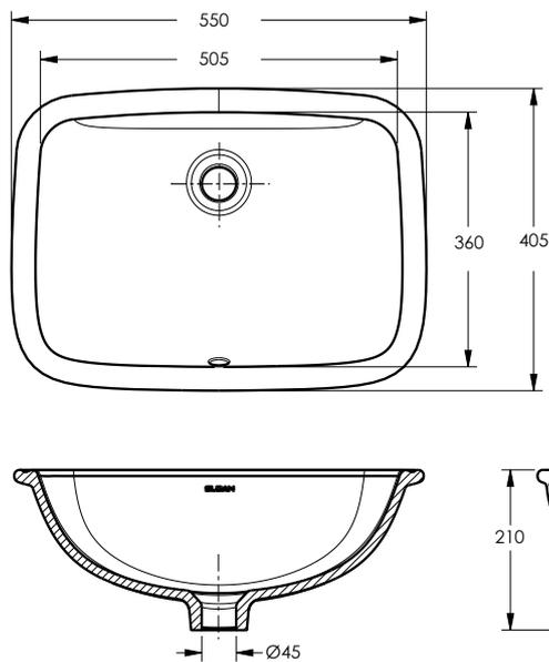
**Note:-**All vitreous china dimensions shown in these drawings are nominal. Dimensions can vary within the tolerances established in the governing BIS standard. Please take this into consideration when planning rough-in and plumbing layouts. Product illustrations shown are representative only; actual products may vary. Sloan reserves the right to make changes in product characteristics, packaging or availability at any time without notice.
