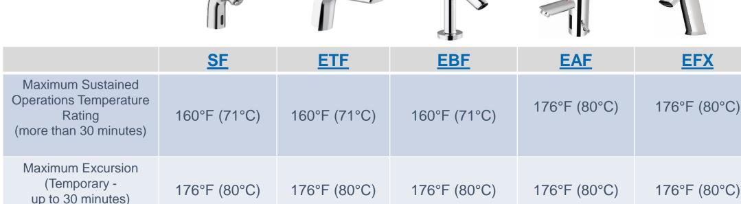
All Sloan Automatic Sensor Faucets can accommodate recommended "Superheat and Flush" Thermal Disinfection Requirements of 160°F - 170°F (71°C - 77°C) while continuously flushing each outlet in a system for at least 30 minutes and up to 120 psi (827 kPa)
