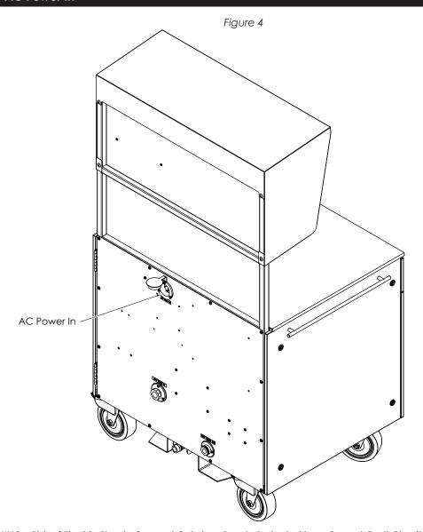
WARNING - Risk of Electric Shock. Connect Only to a Supply Protected by a Ground-Fault Circuit-Interrupter (GFCI).
