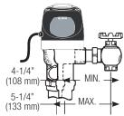
Maximum adjustment of Sloan Adjustable Tailpiece is 1/2" (13 mm) IN or OUT from the standard 4-3/4" (121 mm) (Flushometer centerline to Control Stop centerline). If roughing-in measurement exceeds 5-1/4" (133 mm), consult factory for longer tailpiece.
