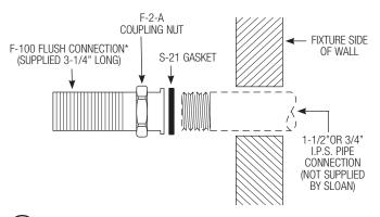
**(B)** Cut Vacuum Breaker and Flush Connection tubes to length.
